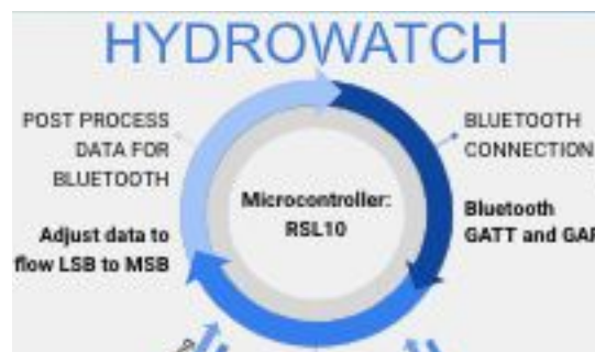
Figure 12. Bluetooth subsystem block diagram
